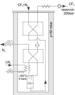
Figure 4: Separation plant for the RICH 1 detector, Figure 5: Separation plant for the RICH 2 an isolated cold box
