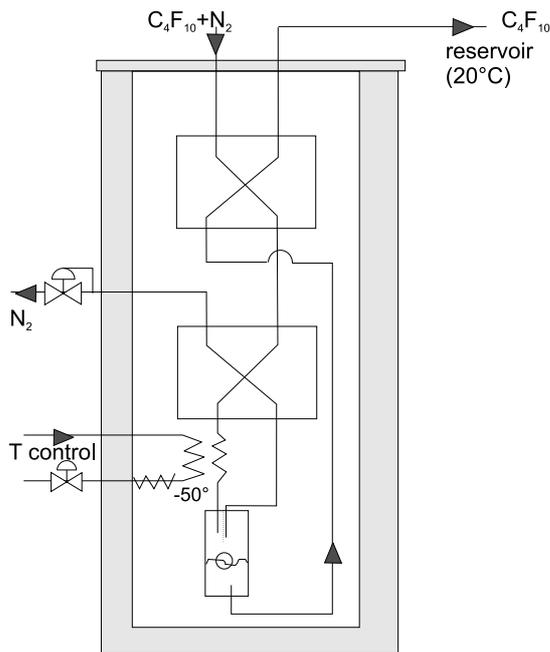
**Figure 4:** Separation plant for the RICH 1 detector, an isolated cold box
